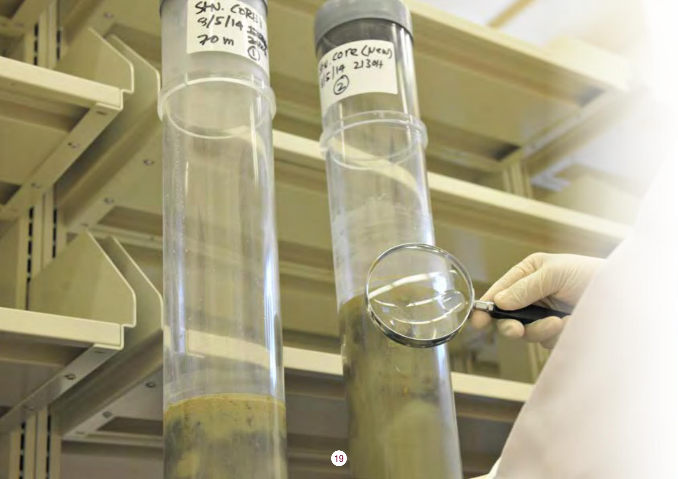
The sediment laboratory conducts particle size distribution analysis for sediments, soils and other particles of different materials using Laser diffraction method, ISO 133320:2009 (E). The laboratory utilizes a Malvern Mastersizer 2000 and Mastersizer 3000 instrument and also has a Test Sieve Shaker to conduct particle size analysis by dry sieving.
